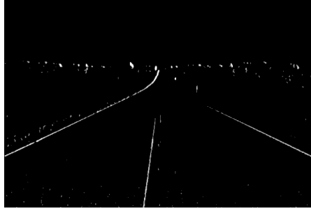
Figure 11: Image from Figure 10 with applied Sobel operator
