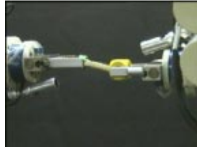
Figure 3: An inconvenient start-situation for screwing
