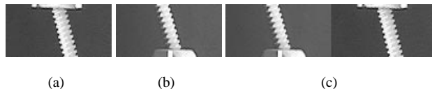
Figure 5: Clipped images from camera 1 (a) and camera 2 (b) and the resulting merged image (c).
