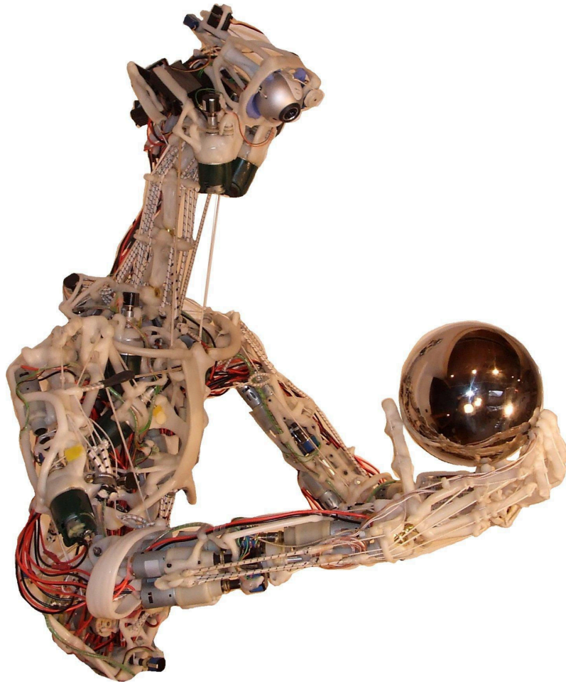
Figure 1.2: ECCE3, the third prototype of an anthropomorphic robot in the ECCEROBOT project. It consists of a torso, head and two arms and is actuated by 60 artificial muscles.
