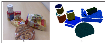
Fig. 1. Primitive Shape Decomposition example : (a) original Point Cloud (b) result of Primitive Shape Decomposition.
